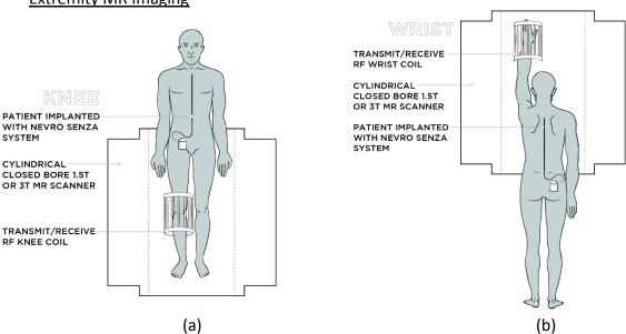
Figure 2: Extremity scans are permissible using an appropriate transmit / receive RF volume coil, as long as the RF volume coil is not placed over the implanted Nevro Senza system
